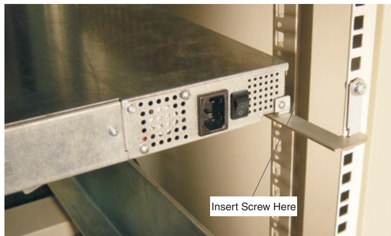
Figure 11. Attaching the autoloader to the rails
