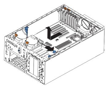
12. Push the system-board release latch toward the side of the system board where the DIMM slots are located to release the board.
