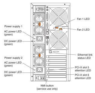
**Fans 1 and 2 LEDs:** These LEDs provide status information about rear fans 1 and 2. For additional information, see "Light path diagnostics" on page 38.
