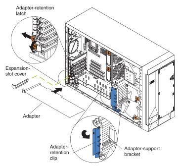
Complete the following steps to install a hot-plug PCI or PCI-X adapter:
