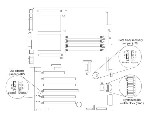
Table 6 describes the function of each switch on the switch block.
