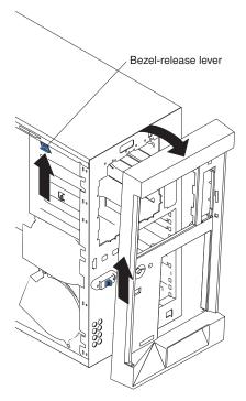
Complete the following steps to remove the bezel:
