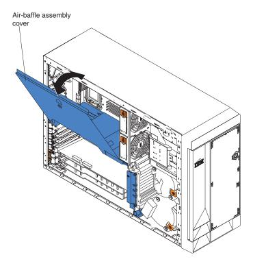
Note: It might be easier to turn the server on its side and remove the air baffle to access the microprocessors.
