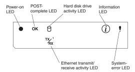
Important: If the power-on LED is off, it does not mean there is no electrical current present in the server. The LED might be burned out. To remove all electrical current from the server, you must unplug the server power cords from the electrical outlets or from the uninterruptible power device.
