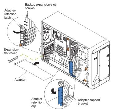
**Attention:** You must install the IXA adapter jumper (J42) between pins 2 and 3 when using an Integrated xSeries Adapter (IXA) in slots 5 and 6 (see "System-board switches and jumpers" on page 51).
