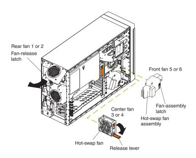
Determine which fan to replace by checking the LEDs on the fans. The front fans, center fans, and rear fans are installed differently from each other. This section contains separate instructions for each group of fans.
