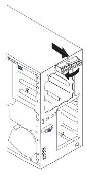
10. Remove the panel, carefully threading the cable past the other components and through the opening in the chassis.
