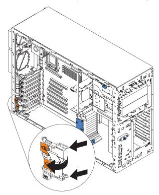
6. Press the two tabs on the hot-swap card and remove it from the chassis.
