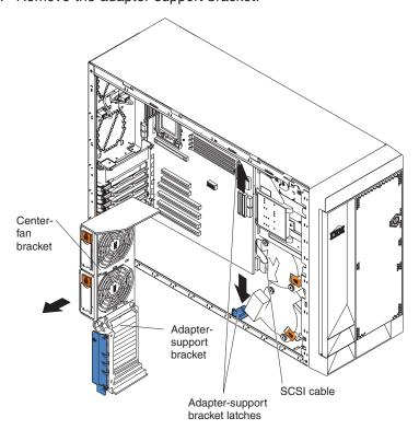
a. Press the release tab on each adapter-support bracket latch. There are two latches; one at each end of the adapter-support bracket.
