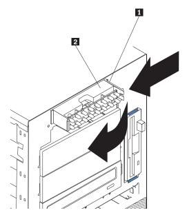
9. From outside the server, push the tab 1 on the panel 2, making sure to press the tab near the chassis; the panel will disengage from the chassis.
