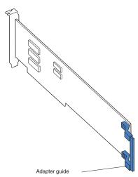
b. Carefully grasp the adapter by its top edge or upper corners, and align it with the expansion slot on the system board.
