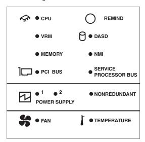
The system-error LED on the operator information panel is lit when certain system errors occur. If the system-error LED on your server is lit, you can check the diagnostics panel to see if any LEDs are lit. You can determine the cause of the error and the action you should take by checking the table at "Diagnostic panel system error LED" on page 132.
