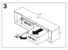
To remove a power supply, grasp the pull-ring on the power supply lever and squeeze to release it; then, pull the lever fully open and remove the power supply from the storage server.
