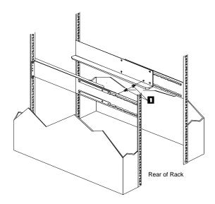
6. Remove the two small 6-32 screws (1) on the interior side of the rails. Save these screws to install the expansion unit.
