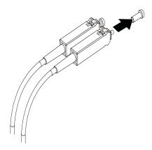
6. Connect the fiber-optic cable to the installed GBIC.
