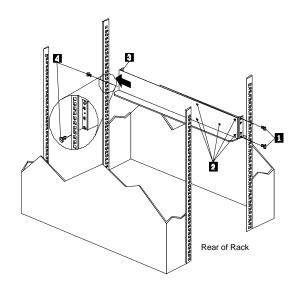
2. Loosen the five screws (four large screws and one small screw) (2) located on the interior of the rail assembly; then slide the front rail assembly forward (3) until it makes contact with the front rack rail.
