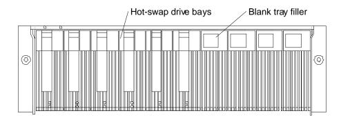
Attention: Never hot swap a drive CRU when its green Activity LED is flashing. Hot swap a drive CRU only when its amber Fault LED is completely on and not flashing or when the drive is inactive with the green Activity LED completely on and not flashing.
