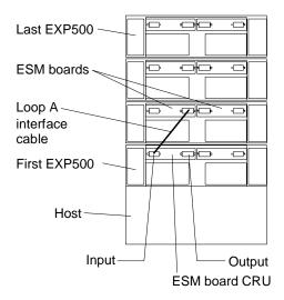
**IBM FAStT EXP500 loop redundancy:** The IBM FAStT EXP500 expansion unit provides redundant loop support. This redundant loop support is available when the second ESM board is configured (as shown in the following figure). If an ESM board, cable, or GBIC fails on a loop, the second loop provides an additional measure of redundancy (that is, an alternative path to your disk drives).
