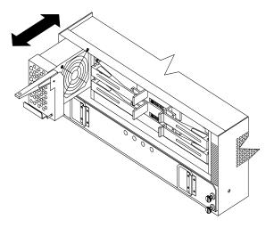
b. Unlock and open the controller levers; then, using the levers, pull the controller out a couple of inches. Grasp both sides of the controller and remove it.
