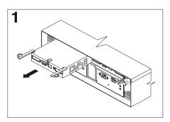
To remove a RAID controller, push down on the latch centered above the controller; then, grasp the pull-rings on the levers and pull them to remove the RAID controller and set it aside for later installation.
