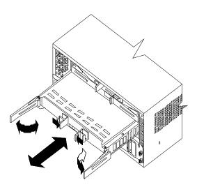
Note: Keep track of which controller CRU belongs in each slot. To prevent data loss, you must replace each controller (A or B) in its original slot.
