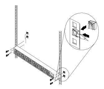
If the rack has square holes, use the M6 clip nuts and hex washer headed screws. If the rack has round holes, use the 10-32 clip nuts and hex washer headed screws.
