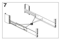
Tighten the rail adjustment screws 1 on both
