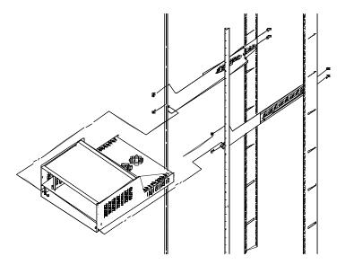
Before removing or placing the controller unit in the rack, carefully remove the battery from the controller unit. See "Replacing the battery" on page 98.
