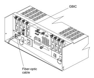
2. Remove the GBICs from the mini-hub ports. If the GBIC you are removing has a metal latch, move the latch to the unlocked (center) position. Pull the failed GBIC from its mini-hub port.
