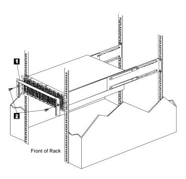
2. Remove screws (2) and remove bezel (1).
