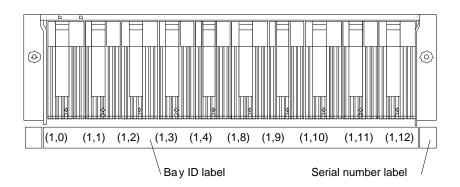
If the two channels are daisy chained using option switch 1 in the off position and switch 5 is on (for tower orientation), then the SCSI IDs are as shown and the drives are all on the same channel.
