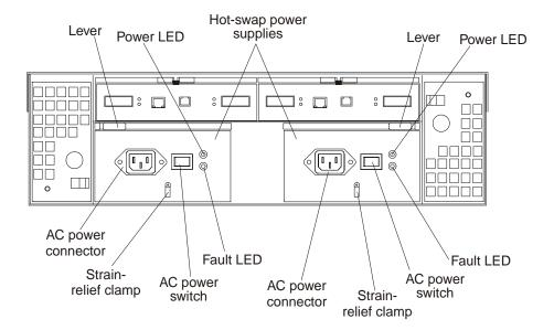
**Levers** Use these locking handles to remove or install a power supply.
