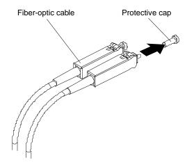
2. Connect the fiber-optic cable to a GBIC that is installed in a mini-hub.
