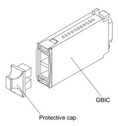
2. If the GBIC you are installing has a metal latch, move the latch to the unlocked (center) position. Slide the GBIC into the port; then, rotate the latch outward to the locked position (flush with the rear of the GBIC).
