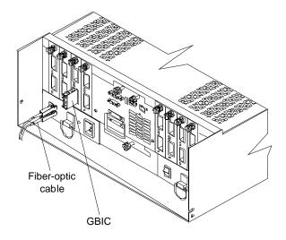
3. Insert the protective cap on the GBIC.
