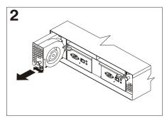
To remove a hot-swap fan, slide the latch on the fan to unlock it; then, pull the handle and remove the fan from the storage server.
