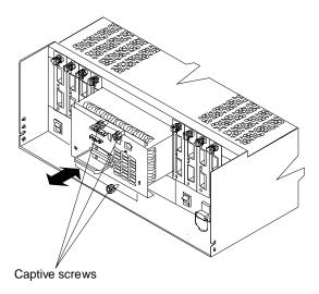
d. Loosen the captive screws; then, grasp the screw and pull the mini-hub from the chassis.
