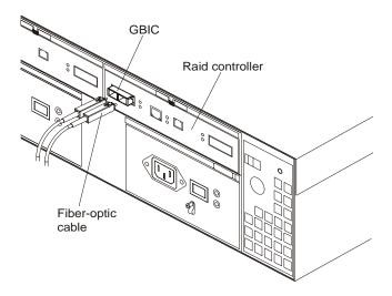
The fiber-optic cable connection is keyed for proper insertion.
