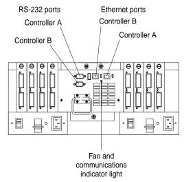
4. Remove the failed fan and communications CRU from the controller unit.
