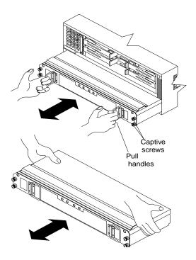
Using the pull tab handle, lift up and pull to release each power supply; then, slide out the power supply.
