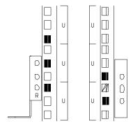
Note: Use clip nuts if your rack has round holes. If your rack has square holes, you can use the rack insertion tool or a flat-blade screwdriver to install cage nuts.
