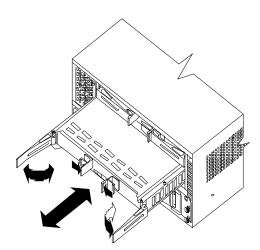
Attention: To avoid potential data loss, make sure that the new controller has the same memory size as the one you are replacing. If you install a controller with a different memory size, the storage-management software suspends cache mirroring and issues an error message. If the memory size is not the same, you need to upgrade the cache memory. For more information, see "Installing additional cache memory in a controller" on page 128.
