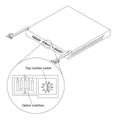
SCSI bus and ID settings: When you install a drive CRU in the expansion unit, the drive tray plugs into a printed circuit board called the midplane. The midplane sets the SCSI bus number and ID automatically, based on the setting of Option Switch 1 and the physical location (bay) of the drive CRU.
