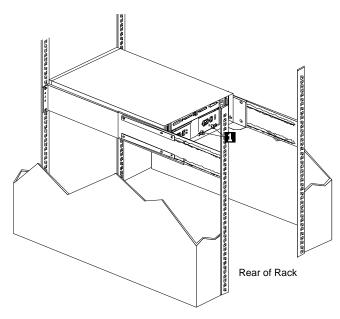
1. Remove screws (1) from assembly rails at rear.
