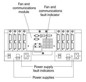
The storage-management software causes the fault indicator to light before the temperature has risen sufficiently to shut down the power supplies. The light comes on when the controller unit temperature exceeds 45° C (113° F). The controller unit shuts down if the temperature rises to 70° C (158° F). If both power supplies shut down, the fault indicator cannot come on.
