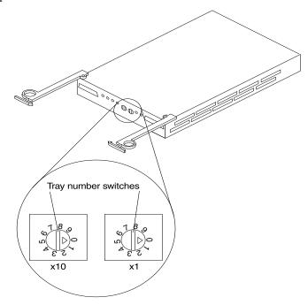
Fibre Channel (FC) loop and ID settings: When you install a drive CRU in the expansion unit, the drive tray plugs into a printed circuit board called the *midplane*. The midplane sets the fibre channel loop ID automatically, based on the setting of the tray number switch and the physical location (bay) of the drive CRU.
