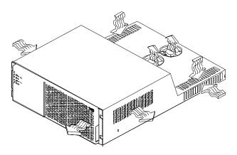
The controller unit must have proper air circulation throughout the chassis. To boost air circulation, the chassis has air vents along its top and sides. These vents serve as air intake and exhaust passages. Assure that vents are clean and free of obstruction.
