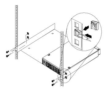
If the rack has round holes, slide the 10-32 clip nuts into place on the rear of the rack.
