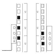
**Note:** Use clip nuts if your rack has round holes. If your rack has square holes, you can use the rack insertion tool or a flat-blade screwdriver to install cage nuts.
