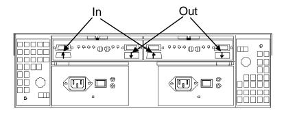
**Note:** In the figure above, the connections for the GBICs are labeled as "In" and "Out." This designation of the connections is for cabling routing purposes only, as all Fibre cables have both a transmit fiber and receive fiber in them. Any connection can function as either output or input (transmitter or receiver).
