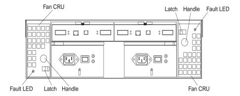
**Fan CRUs** The two fan CRUs are hot-swappable and redundant.
