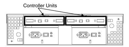
The following figure shows a configuration containing both controllers. It uses GBICs for the connection but does not have the mini-hub feature of the 3552. There is a place for a single host to attach to each controller without using an external concentrator. The other connection on each is used to attach more drives via EXP500 enclosures.
