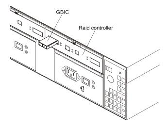
4. After the GBIC is inserted into the port completely, rotate the GBIC latch outward to the locked position (flush with the rear of the GBIC).
