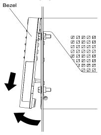
To replace the bezel, slide the top edge under the lip on the chassis; then push the bezel bottom until the pins snap into the mounting holes.
