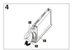
To remove a hard disk drive 2, press the blue latch 3 and pull the handle 1 upwards; then, carefully pull the drive from the storage server.
