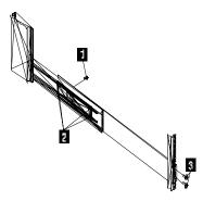
3. Hold the rail against the outside of the left rack mounting flange and loosely insert the front black hex screws (3).
