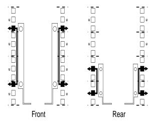
Use clip nuts if your rack has round holes. If your rack has square holes, you can use the cage nut insertion tool or a flat-blade screwdriver to install cage nuts.
