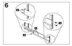
On the rail marked R, remove the 6-32 in. screw 3 and loosen the four screws 2; then, hold the front of the rail against the outside of the right rack-mounting-flange and loosely install two M6 screws 1
