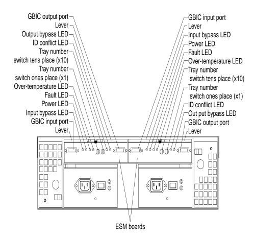
ESM boards The environmental services monitor (ESM) boards contain the expansion unit controls, switches, and LEDs. Each ESM board has two GBIC ports for connecting the expansion unit to the controller.
