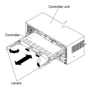
2. Remove both screws from the top cover of the controller; then, lift the cover and set it aside to install after you upgrade your cache.
