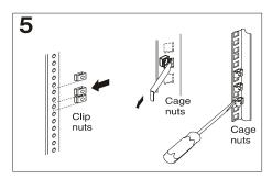
Use the attached template and stickers to mark the appropriate holes on your rack; then, install clip nuts or cage nuts as required for your rack cabinet.
