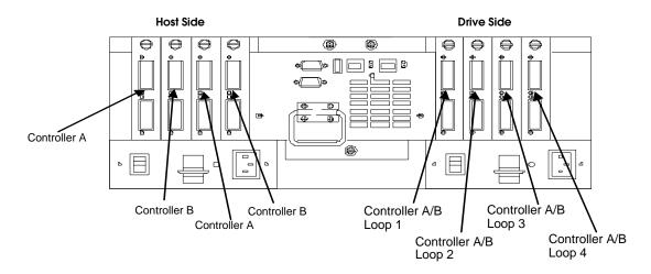
The following figure shows the locations of the controller units in a FAStT200 Fibre Channel controller and drive enclosure unit.
