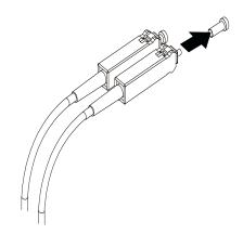
2. Connect the fiber-optic cable to the installed GBIC, as shown in the following figure.
