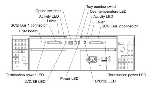
**Note:** SCSI Bus Connectors are 68-pin VHDCI connectors used for attaching SCSI
