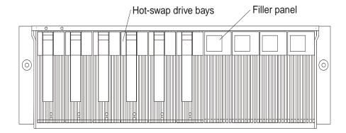
**Attention:** Never hot-swap a drive CRU when its green Activity LED is flashing. Hot-swap a drive CRU only when its amber Fault LED is completely on and not flashing or when the drive is inactive with the green Activity LED on and not flashing.
