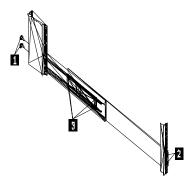
5. Tighten the two front screws (2); then, tighten the four large screws (3). Repeat step 2 through step 5 to install the rail marked R on the right side of the rack.
