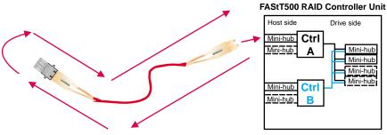
sendEcho path with wrap plug at cable end
