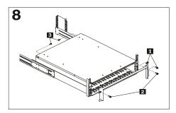
Remove the white screws and nuts 1 from the storage server bezel; then, slide the storage server into the rack. Align the bezel locator pins and attach the bezel with two M6 screws 2; then, install and tighten the 6-32 in screws 3.
