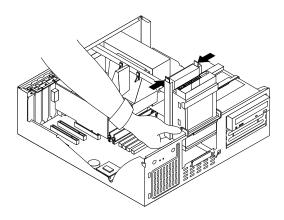
When replacing the drive cage into its horizontal position, be sure place the cage latch back to its regular horizontal position. This is necessary so that the machine cover will fit properly.
