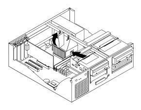
If the air duct does not have a hole, simply swing out the duct to a 45-degree angle and lift it up.
