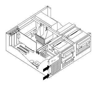
Locate the right tab that hinges the fan/speaker bracket to the chassis. Push the tab to detach the bracket from the chassis.
