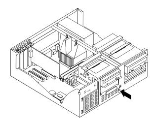
3. Swing the 3.5" drive cage up and latch into vertical.
