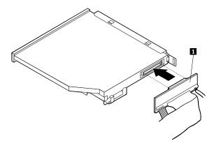
Install the cable and replace the retaining lever behind the CD-ROM.
