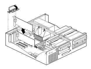
Install the adapter slot cover latch. Pivot the latch back to horizontal
