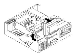
4. Lift the fan/speaker bracket back and out.
