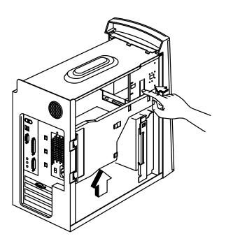
Remove the power supply bracket from the system.
