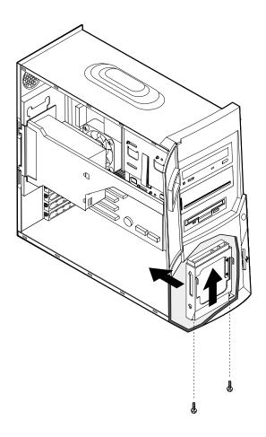
Remove the screws located on both sides of the drive.
