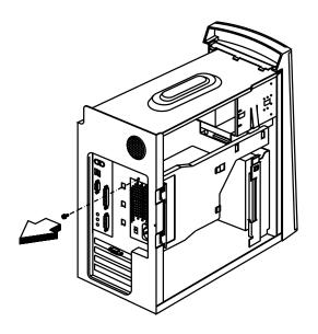
Release the latch secured the bracket.
