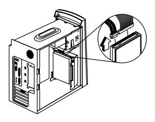
• Remove the two screws that secure the drive cage; then pull up and remove the drive cage from the computer as shown.
