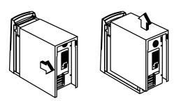
**NOTE:** To prevent the tower from tipping over, you may want to lay the tower on its side on a work surface, such as a table.
