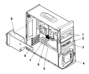
This computer system has four bays that can hold 5.25-inch and 3.5-inch drives. Additional devices can be installed in the empty bays.
