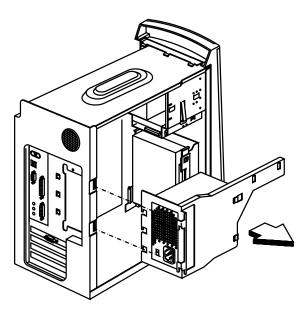
• Remove the four screws in the bracket. Pull out the power supply gently.
