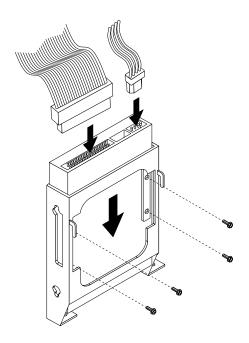
Reinstall the drive cage back into place.
