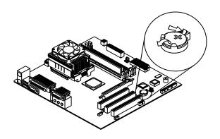
**IMPORTANT:** Make sure to insert the battery with the positive side facing up. A plus(+) sign indicates the positive side.
