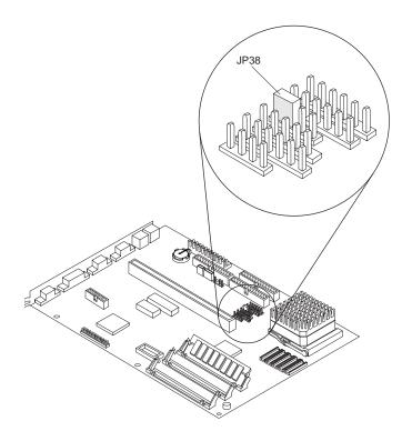
**2.** Lift the jumper from Position 1, move it to Position 2. See the *example*.
