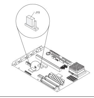
**2.** Lift the jumper from its current position (this could be Position 1 or Position 2). If the jumper is currently in Position 1, move it to Position 2. If the jumper is currently in Position 2, move it to Position 1. See the *example*.
