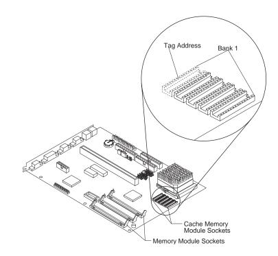
To insert a cache memory module, position the notched end of the module as shown. Align the module pins and insert the module into the socket. Use the individual instructions that follow to install 128K of cache memory.
