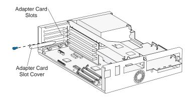
Align and insert the adapter card into the adapter card connector. Insert the screw.
