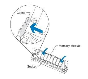
**3.** Lift the module straight out of the socket.
