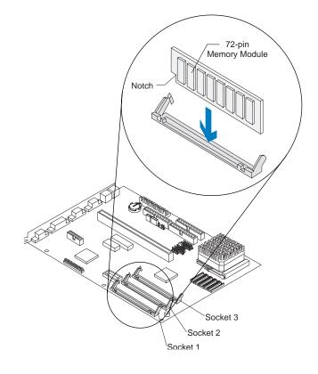
**3.** Press back *firmly* on the memory module until both sides *click*, locking into place. The newly installed memory module will be at an angle with pins showing through the holes on each side.
