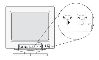
Most monitors have symbols next to the controls that identify the control function.
