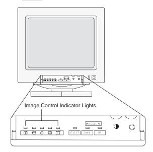
If the monitor cable is disconnected from the note: system unit, the lights next to the symbols will flash consecutively.
