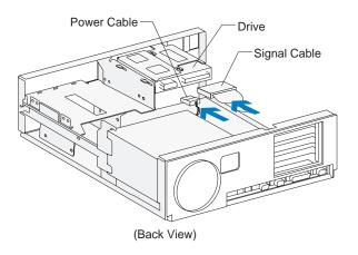
note: If you are adding a diskette or tape drive that attaches to the Diskette connector, make sure the signal cable you plug into the drive is attached to the Diskette connector on the system board. To identify the Diskette connector, see "Identifying parts of the system board" on page 104.
