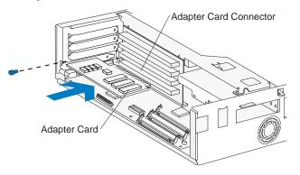
After making hardware changes, reinstall any adapter note: cards you removed and all necessary screws. Reconnect the cables, if necessary.
