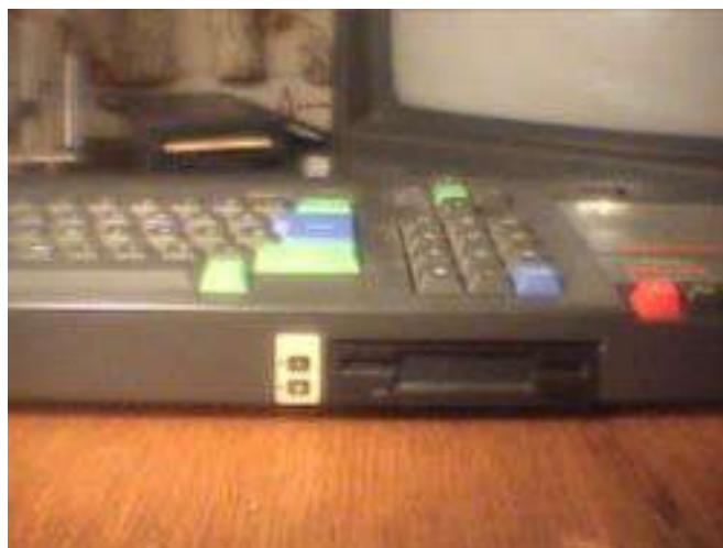
FRONT OF CPC SHOWING INSTALLED DISK DRIVE ALONG WITH A DIGITAL SIDE SWITCH.
