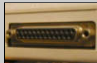
STANDARD PARALLEL CONECTOR AS USED IN THE PC.
