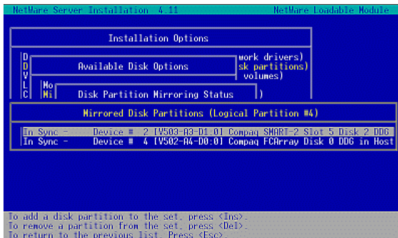
Figure 16 – NetWare Server Installation – Mirrored Partitions
