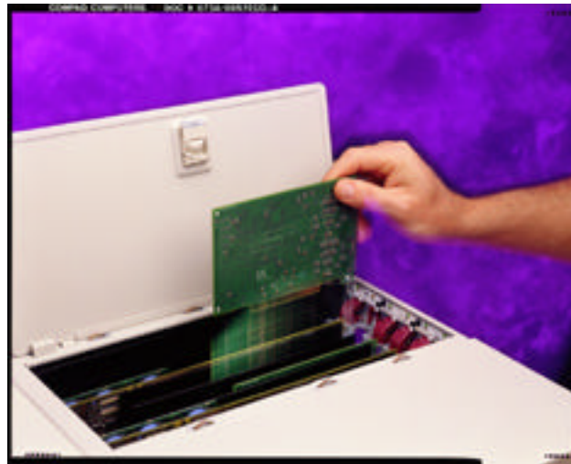
Figure 6. Tool-free access door enables quick replacement of hot-plug aware PCI adapters.
