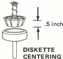
DISKETTE CENTERING Clutch mechanism pro- vides most accurate diskette positioning (within .0008) and longest diskette life.
