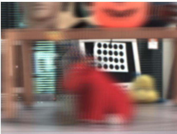
Figure 19: Finally, the focal plane is at the back of the room, making the monitor in focus, while the fish and red bull are blurry.
