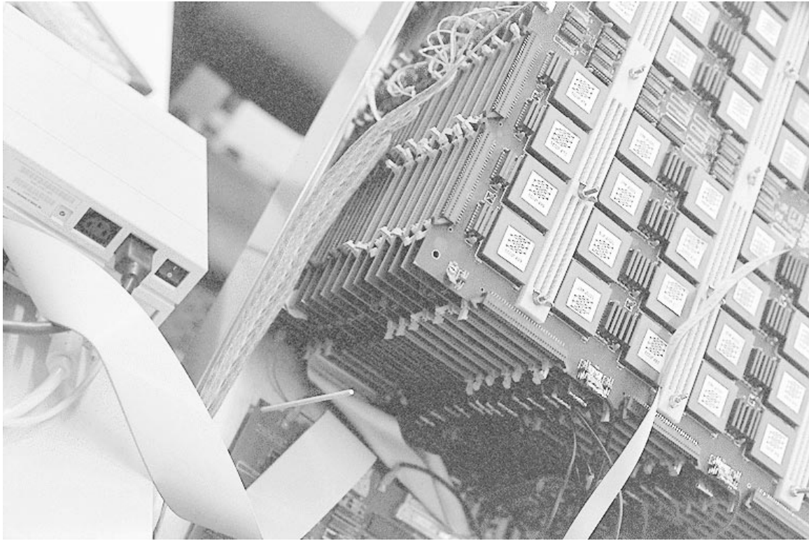
Figure 2-2: Detail photo of the J-Machine with the cover removed which shows some of the individual processors arranged in an array on the top board. Three DRAM chips are next to each processor and are the external local memories; otherwise all of the functional modules of each MDP – the processor, internal memory, queues, routers, control – are on-chip. Processors are wired to their nearest neighbor in the X and Y dimensions through the printed circuit board. The connection in the Z dimension is through elastomeric connectors which are compressed by tightening the pictured wing-nuts onto the shafts which skewer the stack of boards. The unwired network connections on the edge of the cube go to the connectors on the edges of the boards; a ribbon cable from one of these connectors to the host interface card appears at the bottom of the stack.
