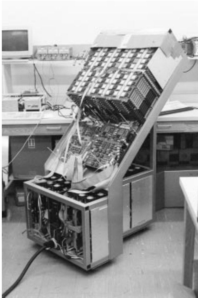
Figure 1-1: Photograph of the MIT J-Machine with the cover removed. The processor are arranged on a stack of 16 printed circuit boards, with each board holding an 8 by 8 array of Message-Driven Processors. You can see this stack in the upper portion of the pictured machine.
