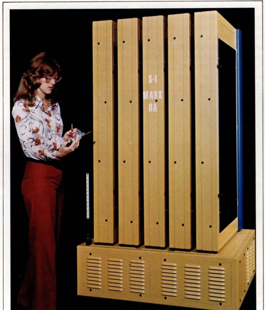
Fig. 4 The S-1 Mark IIA Uniprocessor. The package consists of identical pages. The pages unfold to expose all wire-wrap pins for maintenance. Ambient air blows up through the centers of the pages to cool the integrated circuits, which are mounted on the inside. Commercially available power supplies are mounted in the cabinet base.
