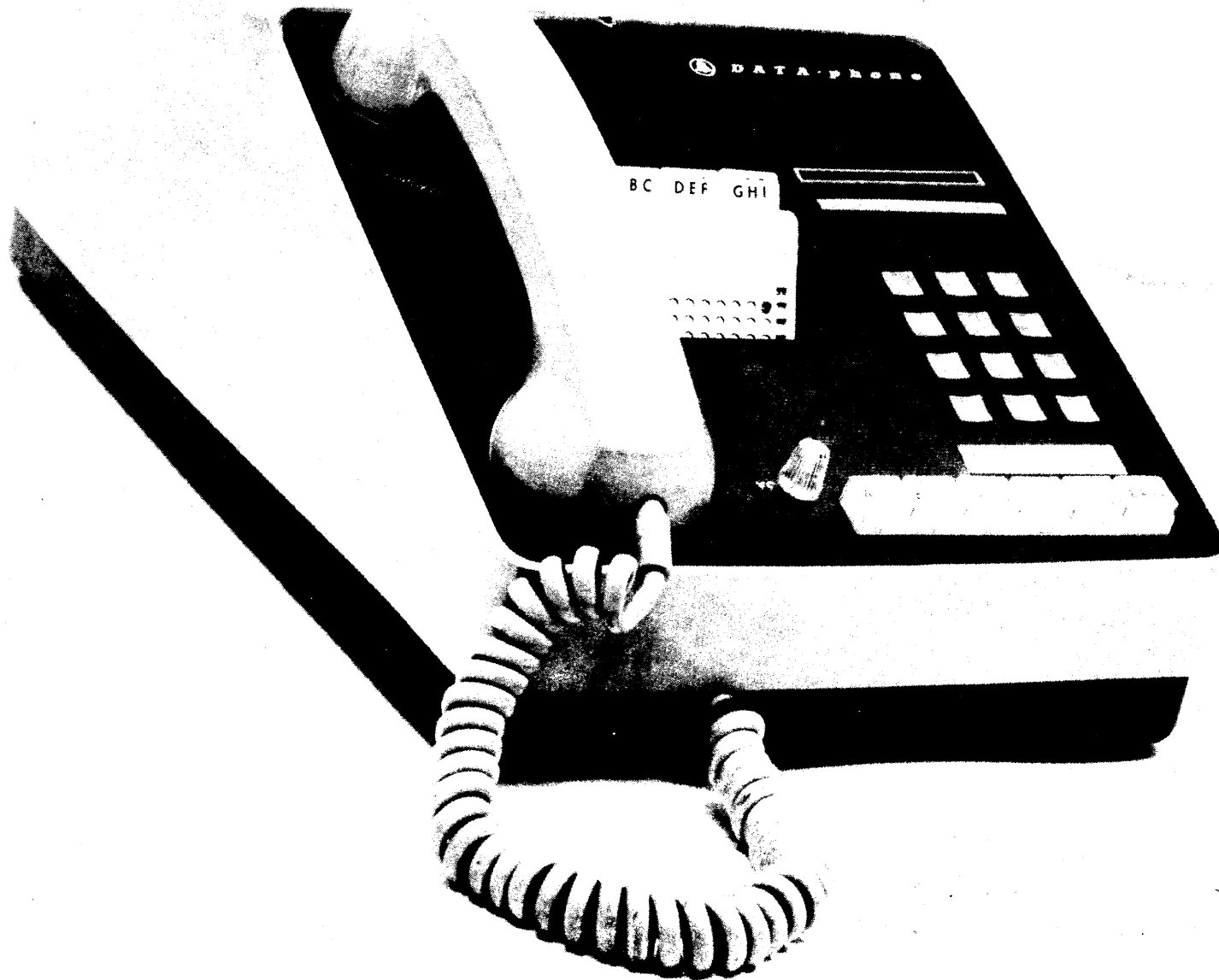
FIGURE 2 DATA SET TYPE 103G WITH TOUCH-TONE DIAL CARD DIALER
